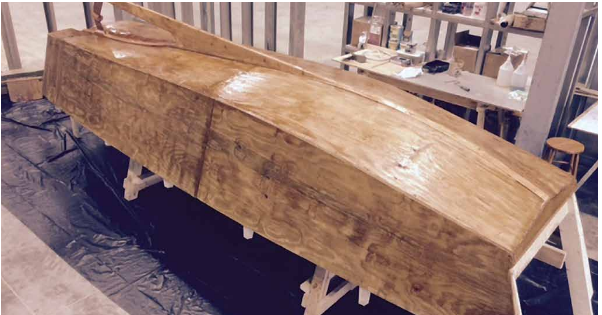
▲ View from the Stern after the first coat of Epoxy
