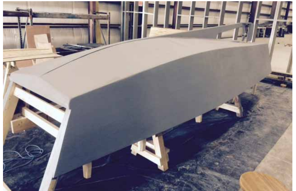
▲ The hull following the first coat of primer.
