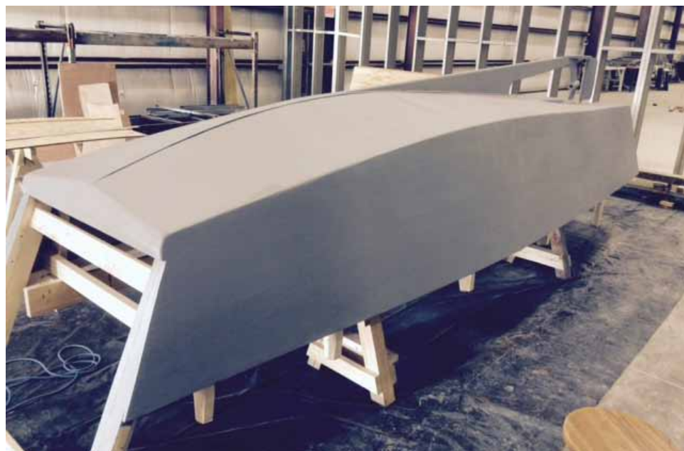
▲ The hull following the first coat of primer.
